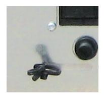
**Room thermostat:** the room thermostat detects the present temperature in the room. When it detects the set temperature on the display, the stove will go into operation in ECO ie hold function to save fuel. The room thermostat should be spread so as not to be conditioned by the temperature of the body stove.
