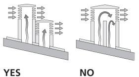
Fig. 5: Characteristics of chimney
