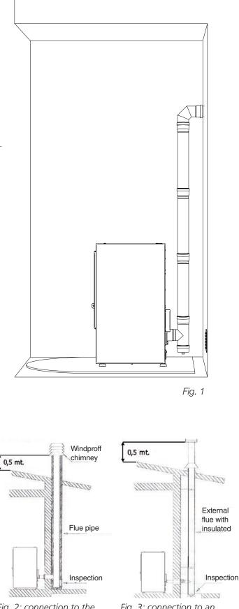
*Fig. 2: connection to the flue pipe.*
