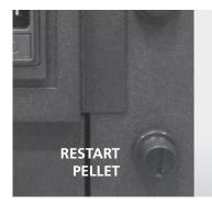
**Pellets temperature safety:** In the rare event there is a too high temperature in the tank, the thermostat for pellets safety with manual reset creates an alarm "*ALAR-SIC-FAIL*" stopping the pellet boiler stove. You need to reset the system working on the device placed on the back of the thermostove.
