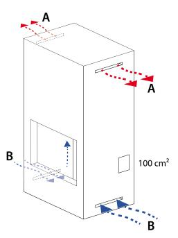
**A** : Air outlet. Minimum section 175 cmq. **B** : Air intake. Minimum section 120 cmg
