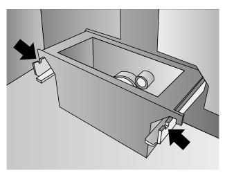
flap for pellets fall (Pict. 11) must be addressed to the inner part of the combustion chamber.
