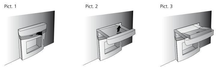
Once you have loaded the pellets, lift the tray so that all the pellets go to the pellet tank (fig. 5). Close the pellets tray (fig. 6).
