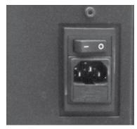
**Electrical safety:** the pellet insert is protected against violent surges of current (ex. lightnings) by the main fuse 4 A which is located on the control panel at the rear of the pellet insert. Other fuses to protect the electronic boards are to be found on the boards themselves.
