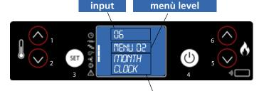
Set the current time and date. The device comes equipped with a lithium battery that allows the internal clock to operate autonomously for over 3-5 years.
