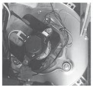
Flue gas temperature sensor: thermocouple that measures the temperature of the fumes while keeping the operation or shuts the pellet insert when the flue gas temperature drops below the preset value.
