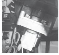
**Reduction motor:** if the motor stops, the pellet insert continues to function until the flame goes out for lack of fuel, and until It has cooled down to the minimum level.
