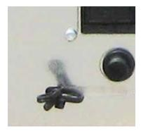
**Room thermostat:** the room thermostat detects the present temperature in the room. When it detects the set temperature on the display, the pellet insert will go into operation in ECO ie hold function to save fuel. The room thermostat should be spread so as not to be conditioned by the temperature of the body pellet insert.
