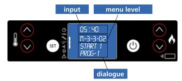
The weekly programmer has 4 independent programmes whose final effect is composed of the combination of the 4 individual programmes. The weekly programmer can be activated or deactivated. Additionally, by setting OFF in the time field, the clock ignores the corresponding command.
