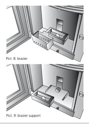
NOTE: when you insert the brazier support, be sure you install it on the stopping device on the support brackets (Pict. 10). The brazier
