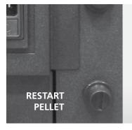
**Pellets temperature safety:** In the rare event there is a too high temperature in the tank, the thermostat for pellets safety with manual reset creates an alarm "**ALAR-SIC-FAIL**" stopping the pellet pellet insert. You need to reset the system working on the device placed on the back of the pellet insert.
